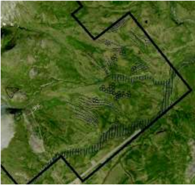
Fig. 3. Fragment of Lik mine site surficial geology map. Cryoplanation terraces (stippled), unfrozen areas (vertical stripes), sorted circles (three circle symbols) and non-sorted stripes (dashed) mapped for the project were easily identified on the computer screen in 3D mode. Unfortunately, the 3D mode cannot be shown on this 2D figure.
