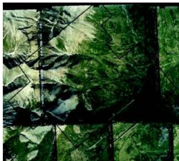
Fig. 2. View of photographic images acquired for the Lik mine site project in northwest Alaska. Black outline shows property boundary, which overlaps 6 stereo photos.
