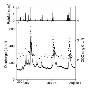
Figure 4 (a) Rainfall amounts and (b) streamflow discharge (solid line) and dissolved organic carbon (DOC) concentration (dots), summer 2001.
