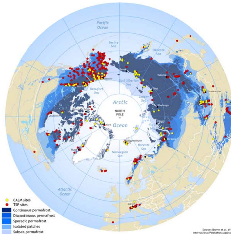
Figure 7: This map shows the sites in the Circumpolar Active Layer Monitoring (CALM) and the Thermal State of Permafrost (TSP) networks. CALM measures active layer thickness and TSP measures permafrost body temperature.
