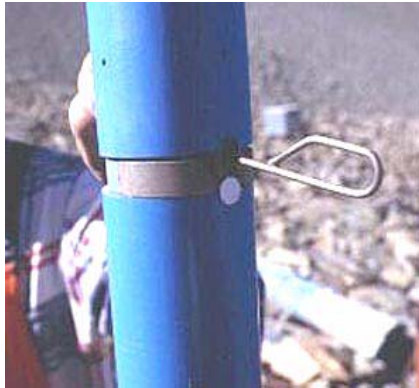
Figure 3-12: Settlement hook system coupling.
