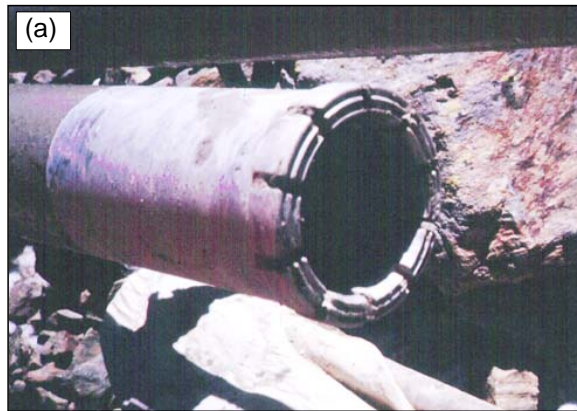
a) diamond drill bit: Seyferle: Type XUPER W2: \varnothing_i = 75 mm, \varnothing_o = 106 mm
