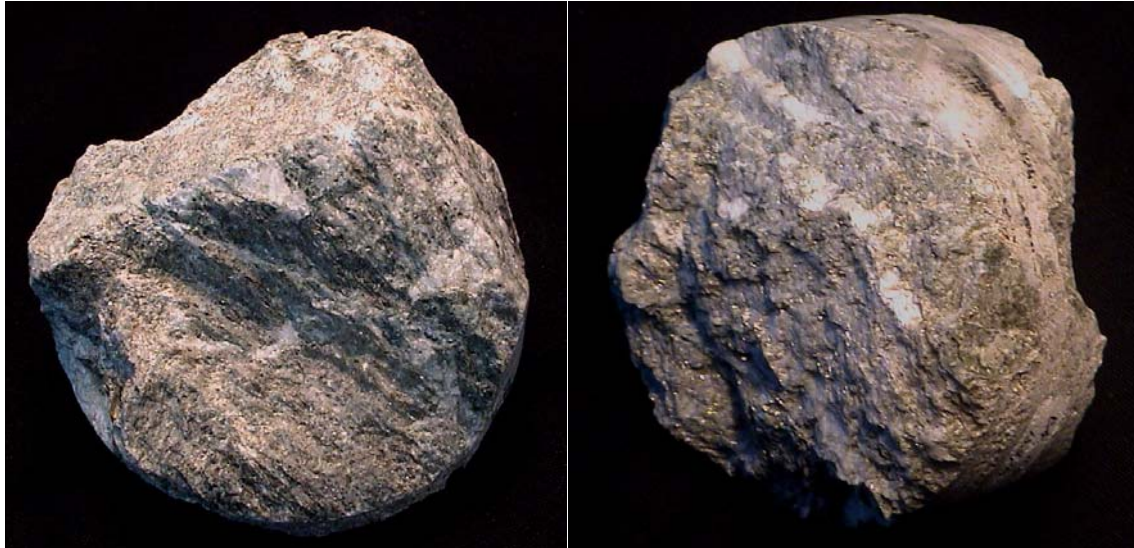
Figure 3-10: Gneissic granite from the Muragl rock glacier at borehole 4/1999, 11.5 m depth, diameter: 75 mm (Photo: L. Arenson).
