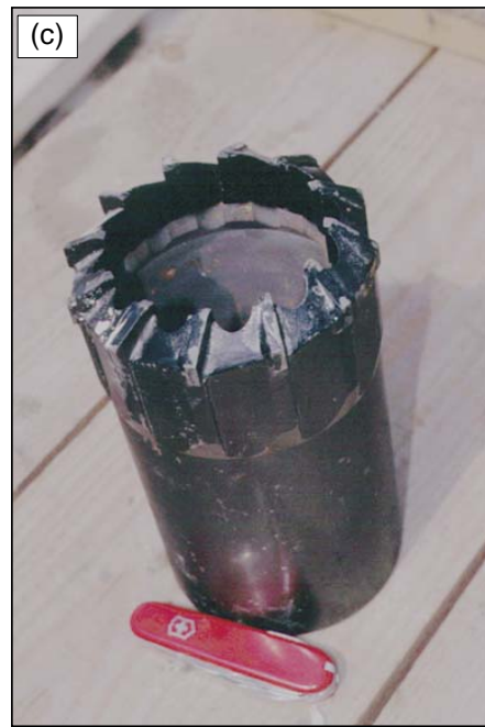
e) drill bit for percussion drilling: \varnothing_o = 90 mm/115 mm
