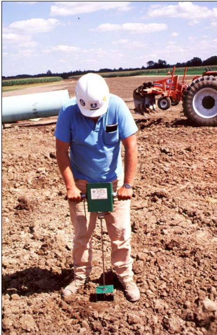
Figure N-7. Environmental inspector (pipelines) conducting soil cone penetrometer testing to verify the efficacy of deep-ripping (sub-soiling) operations in the trench and workspace areas of a pipeline ROW (photo: R.A. McBride).
