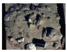
d) Gravelly silty sand till when thawed illustrating high water content
