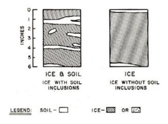
Figure A1 Schematic Description of Ice Inclusions (See subsection 3.5.1)
