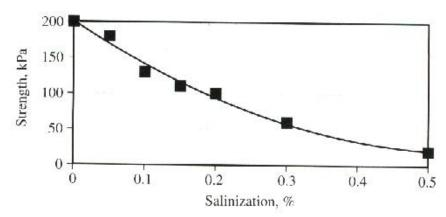
Figure 5 Long-term Strength for Concrete and Marine Sand at -3°C (Brouchkov 2004)
