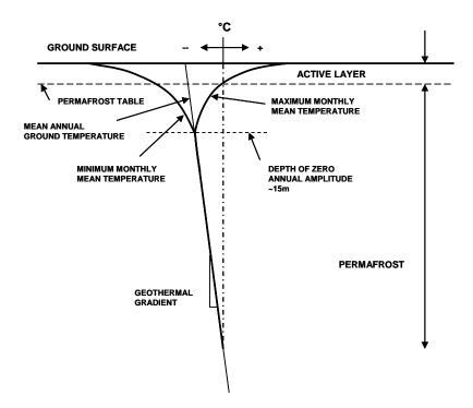
Figure 3 Typical Ground Temperature Regime in Permafrost.
